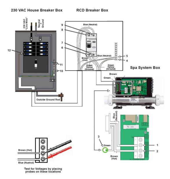
Figure 3. Wiring Schematic for 50 Hz Systems
