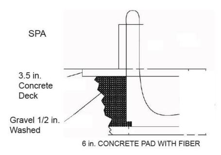
Figure 9. Excavation Cross Section
